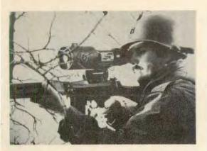
Hyper-Miniscope M9823 mounted on FN/FAL 7.62mm rifle being tested by U.S. Army officer.
